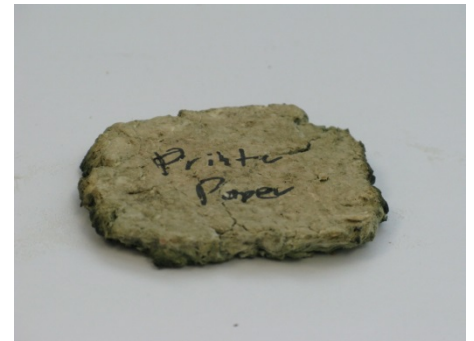
Tough, light-weight composite of recycled paper with algae-cake derived bio-adhesive as binder. May be employed in drywall, ceiling tiles, or similar applications.
