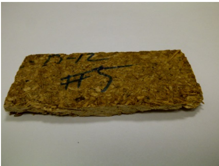
Wood-composite using algae-cake derived bio-adhesive as binder, which may be used as the next generation of paper, particleboard, plywood, or similar materials.
