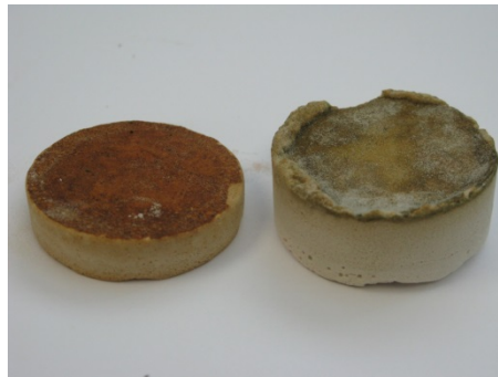
Algae / sand composites which may be used as substitutes for brick, mortar, concrete, asphalt, and other civil engineering applications.
